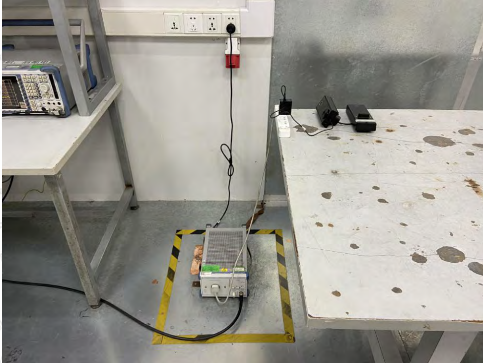
Photo of Conducted Emission Measurement
