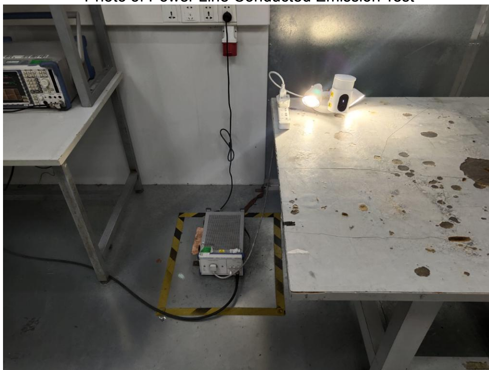
FCC ID: 2AOKB-T8420X Photo of Power Line Conducted Emission Test
