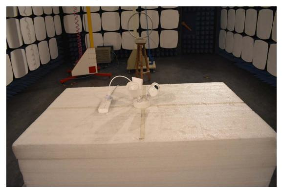
3. Radiated emission (9KHz-30MHz)
