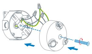
Use the central screw cap to cover the central screw to prevent the central screw from rusting.
