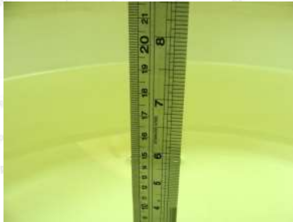
Photo of Liquid Height for Body SAR
