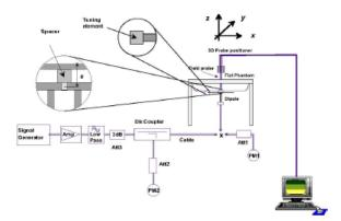
Fig 8.2 System Setup for System Evaluation
