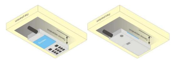
Fig 9.5 Illustration for Body Worn Position
