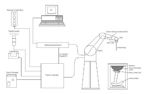
Fig 6.1 SPEAG DASY System Configurations
