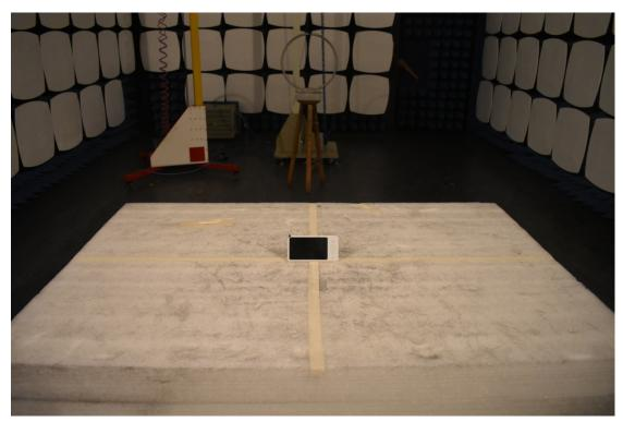
3. Radiated emission (9KHz-30MHz)
