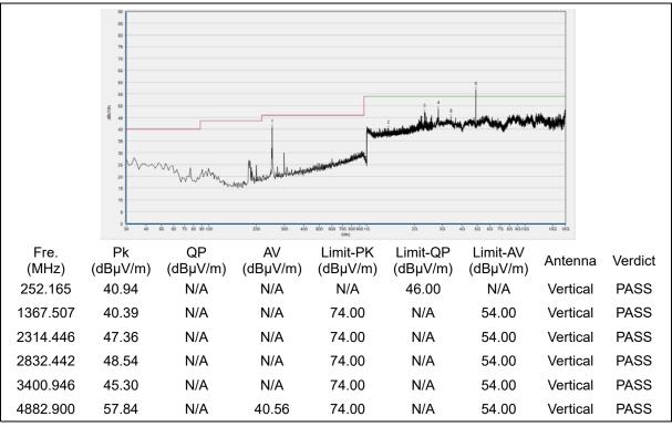
(30MHz to 18GHz, Antenna Vertical, GFSK, channel 10)
