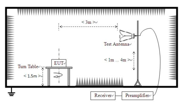
The EUT is located in a 3m Semi-Anechoic Chamber; the antenna factors, cable loss and so on of the site as factors are calculated to correct the reading. For the Test Antenna:
