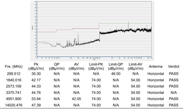
(30MHz to 18GHz, Antenna Horizontal, GFSK, channel 20)
