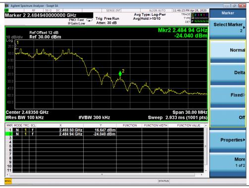
(Channel = 20, Band edge with hopping on, GFSK Mode)
