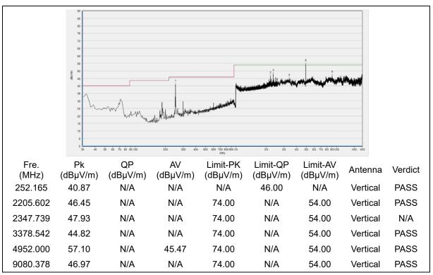
(30MHz to 18GHz, Antenna Vertical, GFSK, channel 20)
