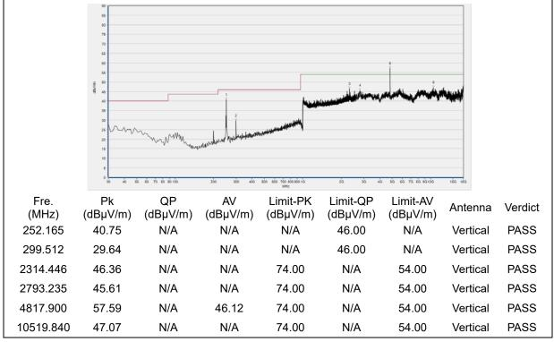
(30MHz to 18GHz, Antenna Vertical, GFSK, channel 1)
