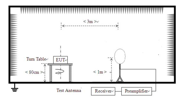
2) For radiated emissions from 30MHz to1GHz
