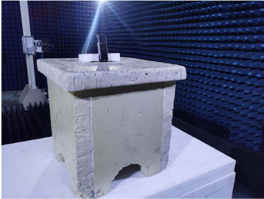
Photo of Radiated Emission Measurement (Above 1G)
