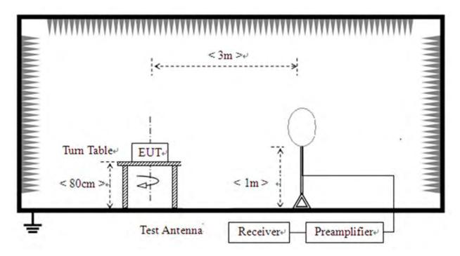
2) For radiated emissions from 30MHz to1GHz
