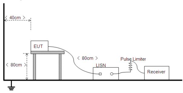
The Table-top EUT was placed upon a non-metallic table 0.8m above the horizontal metal reference ground plane. EUT was connected to LISN and LISN was connected to reference Ground Plane. EUT was 80cm from LISN. The set-up and test methods were according to ANSI C63.10 2013.
