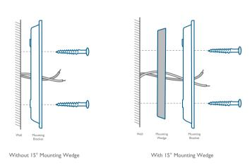
If you're mounting the doorbell on a surface made out of hard materials, like brick, concrete, stucco:
