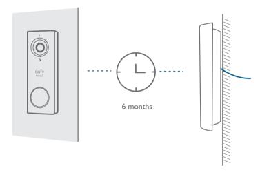
**Note:** The battery life varies depending on usage. In most common cases, a doorbell may have up to 10 events per day and each recording lasts 20 seconds on average. Under this scenario, the doorbell battery life can last up to 6 months.
