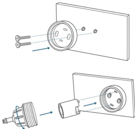
5. Install the solar panel onto its mounting bracket by turning it, then adjust the angle (20°~30° recommended).
