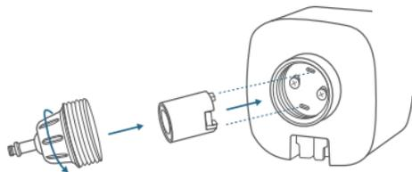
2. Install the solar panel onto the solar panel's mounting bracket by turning it.
