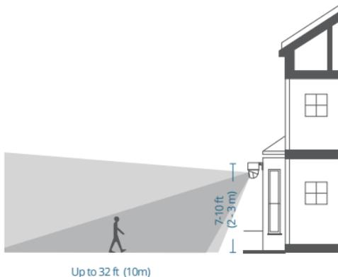
To ensure that no detection is missed, do not install the camera directly facing the monitoring area. Instead, maintain an angle to avoid any potential blind spots.
