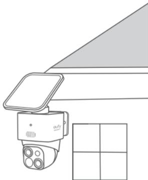
1. Secure the solar panel's mounting bracket to the top of the camera.
