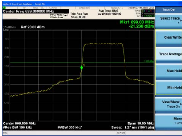
LTE Band 12 16QAM 5MHz CH-Low, 1 RB
