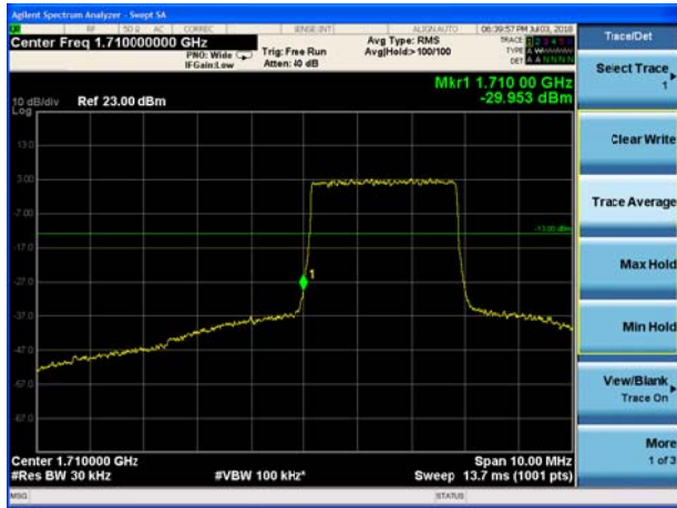
LTE Band 66 16QAM 5MHz CH-Low, 1 RB
