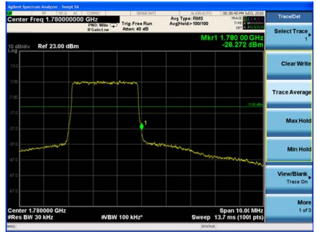
LTE Band 66 16QAM 5MHz CH-High, 1 RB
