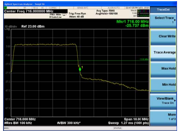
LTE Band 12 16QAM 5MHz CH-High, 100%RB
