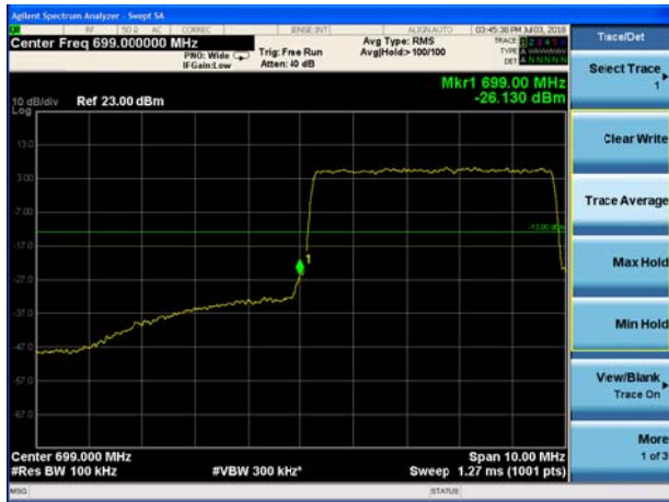
LTE Band 12 16QAM 5MHz CH-Low, 100%RB
