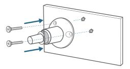
3. Firmly screw the knob of the mounting bracket into the mounting hole of SoloCam.
