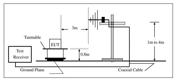
(c) For radiated emissions above 1000MHz
