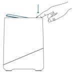
2. Loosen the screw, then pull out the hard drive bracket.
