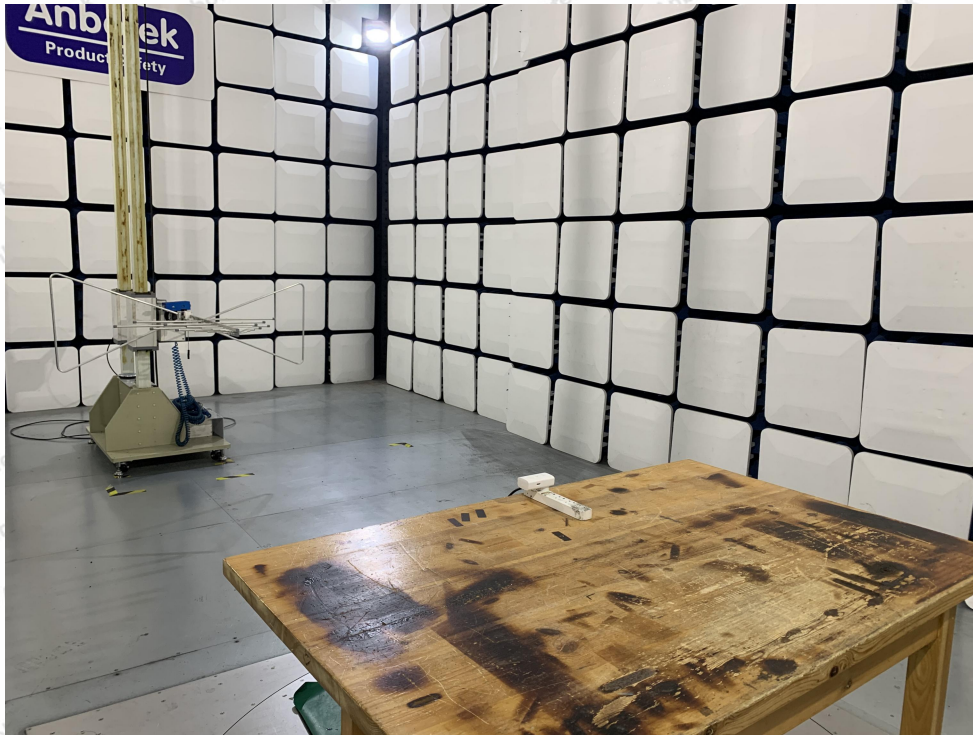
Photo of Radiation Emission Test
