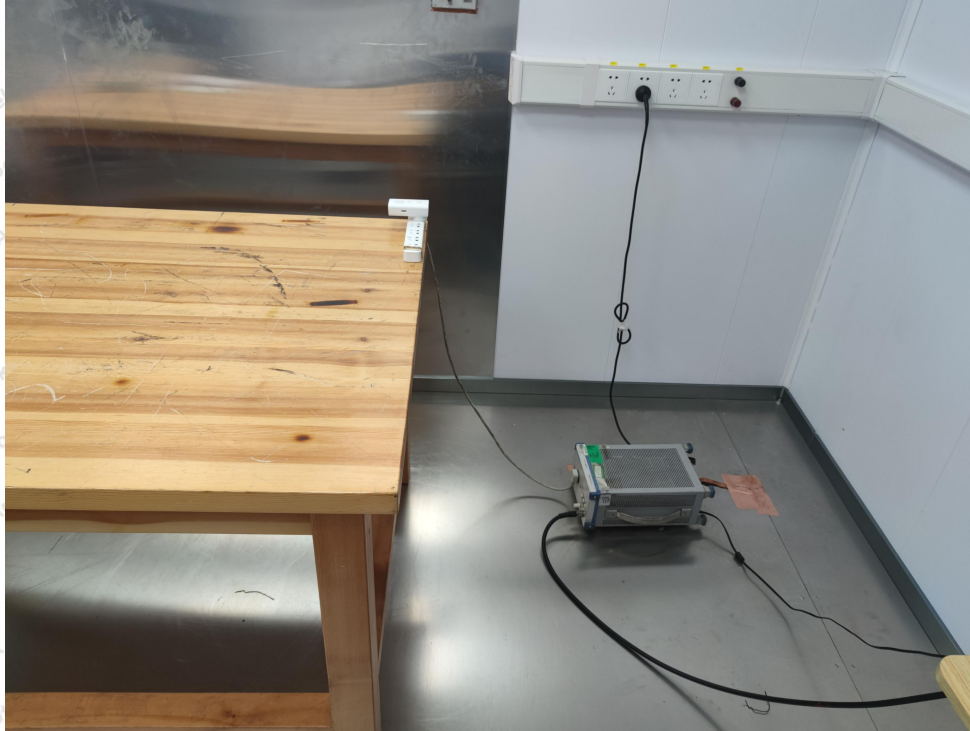
Photo of Conducted Emission Measurement
