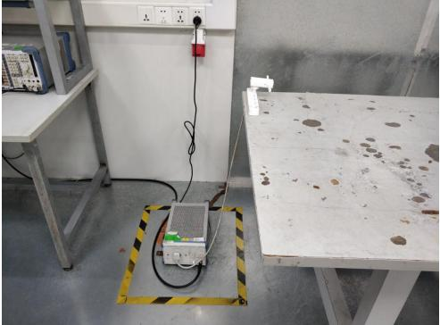
Photo of Radiation Emission Test
