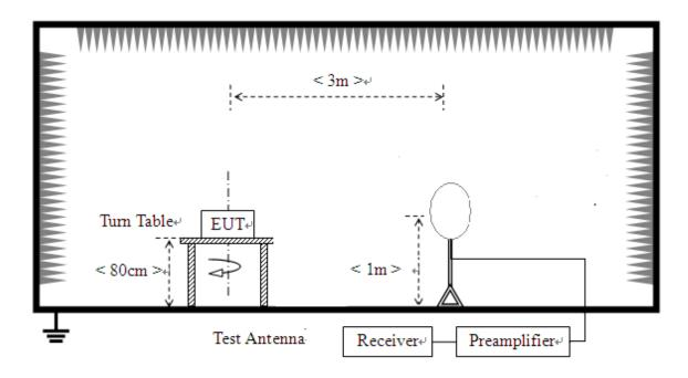
2) For radiated emissions from 30MHz to1GHz
