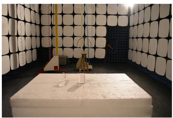
3. Radiated emission (9KHz-30MHz)
