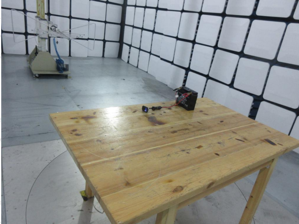
Photo of Radiation Emission Test
