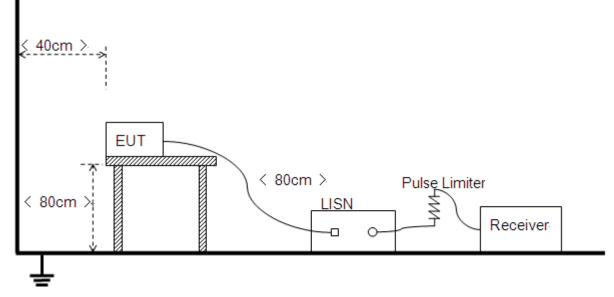
The Table-top EUT was placed upon a non-metallic table 0.8m above the horizontal metal reference ground plane. EUT was connected to LISN and LISN was connected to reference Ground Plane. EUT was 80cm from LISN. The set-up and test methods were according to ANSI C63.10: 2013.
