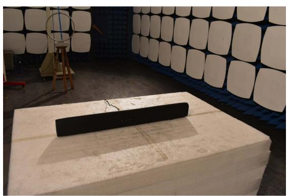
3. Radiated emission (9KHz-30MHz)
