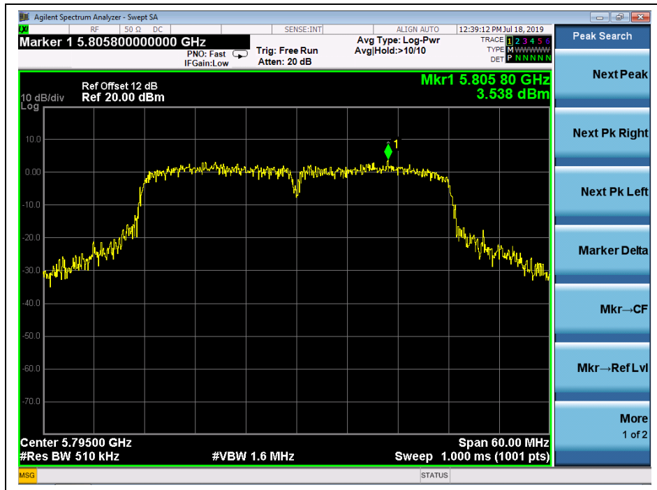
(Channel 159, 5795MHz, 802.11 ac (VHT40))
