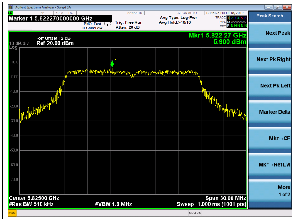
(Channel 165, 5825MHz, 802.11 ac (VHT20))
