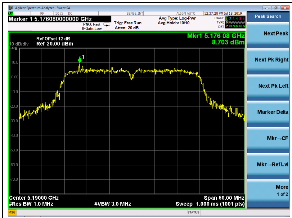
(Channel 38, 5190MHz, 802.11 ac (VHT40))
