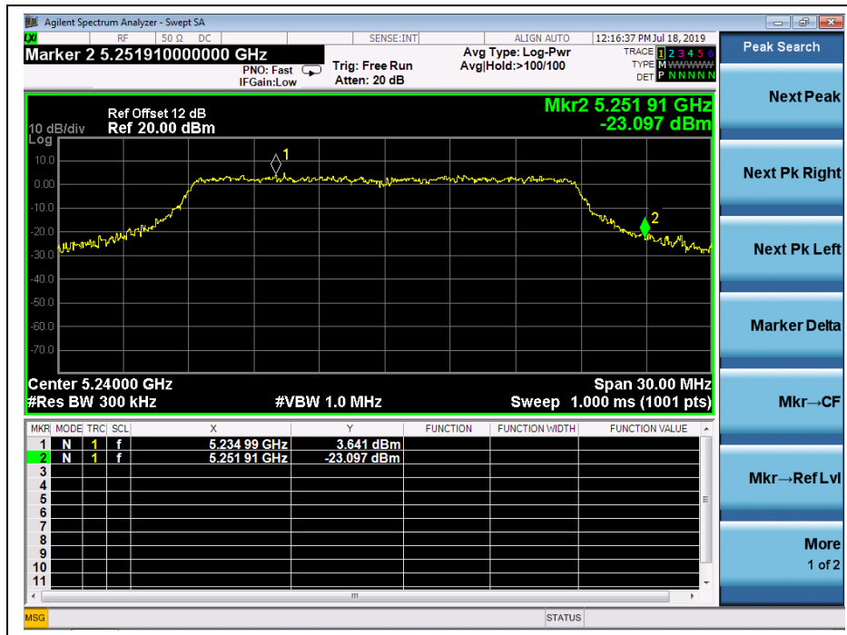
(Channel 48, 5240MHz, fh of -26dB, 802.11 ac (VHT20))
