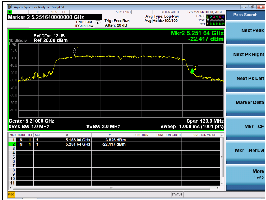
(Channel 42, 5210 MHz, fh of -26dB, 802.11 ac (VHT80))
