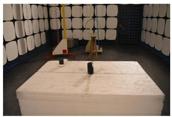
3. Radiated emission (9KHz-30MHz)
