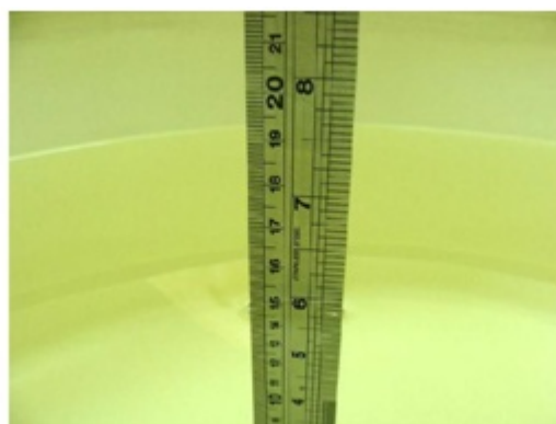
Fig 6.2 Photo of Liquid Height for Body SAR
