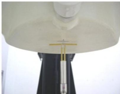
Fig 7.1 Photo of Dipole Setup
