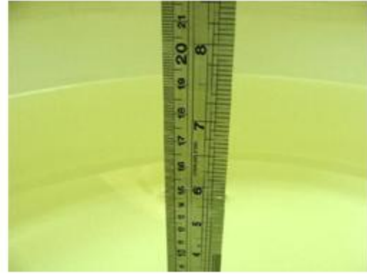
Fig 6.2 Photo of Liquid Height for Body SAR
