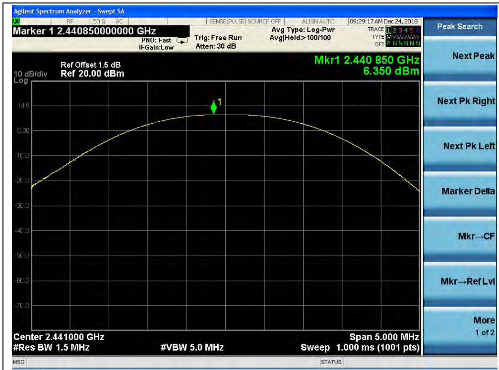
(GFSK, Channel 39, 2441MHz)
