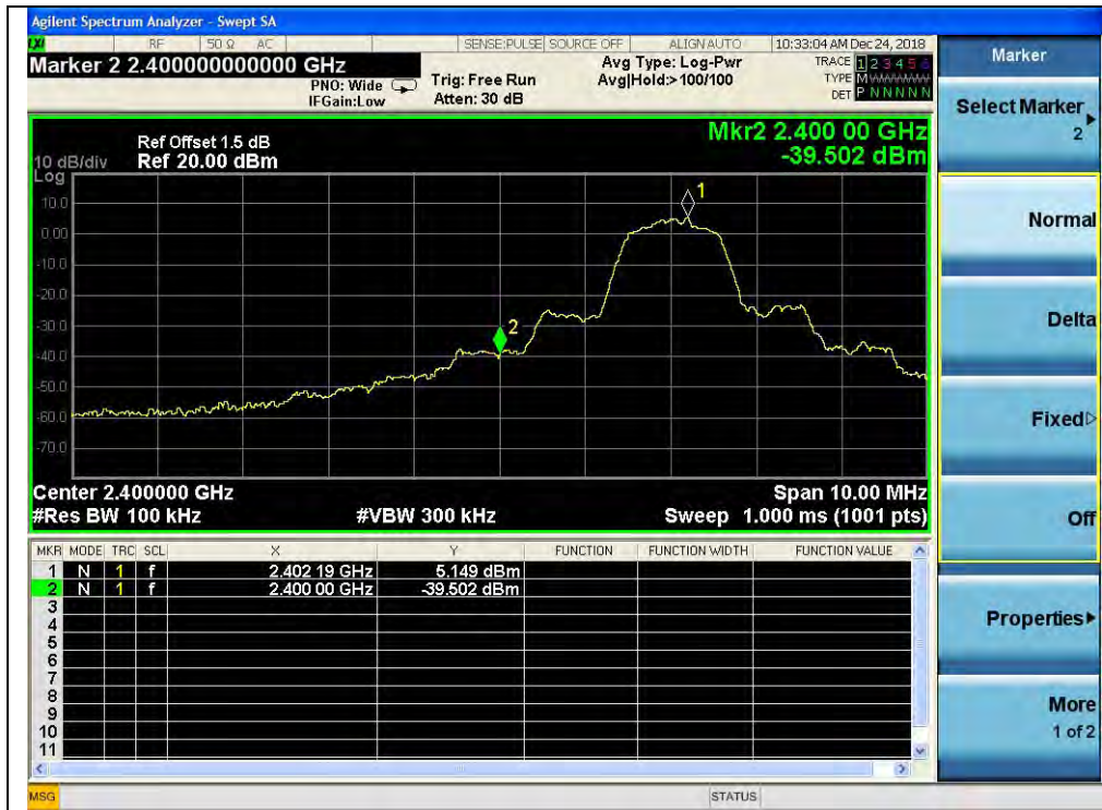
(Channel = 0, Band edge, \pi/4 -DQPSK)
