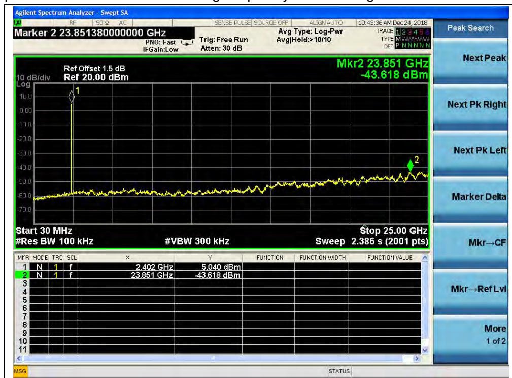
(Channel = 0, 30MHz to 25GH, 8-DPSK)
