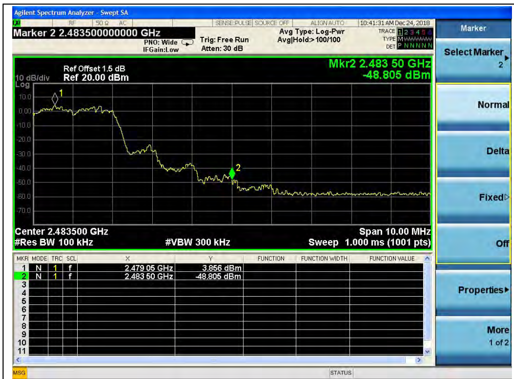
(Channel = 78, Band edge with hopping on, 8-DPSK)
