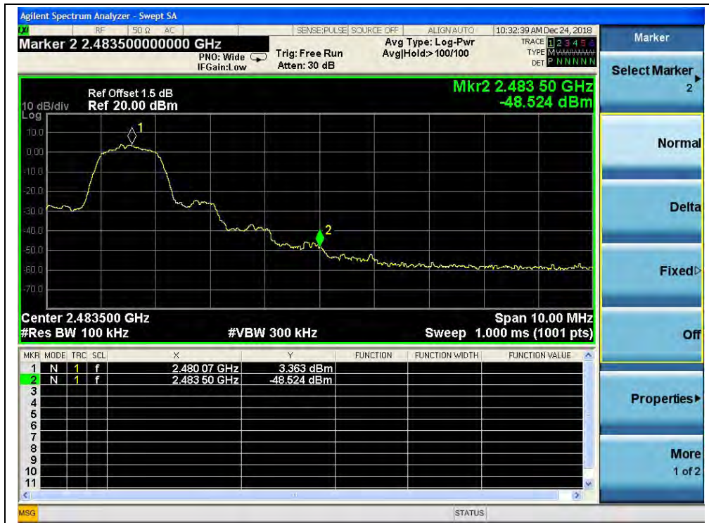
(Channel = 78, Band edge, \pi/4 -DQPSK)
