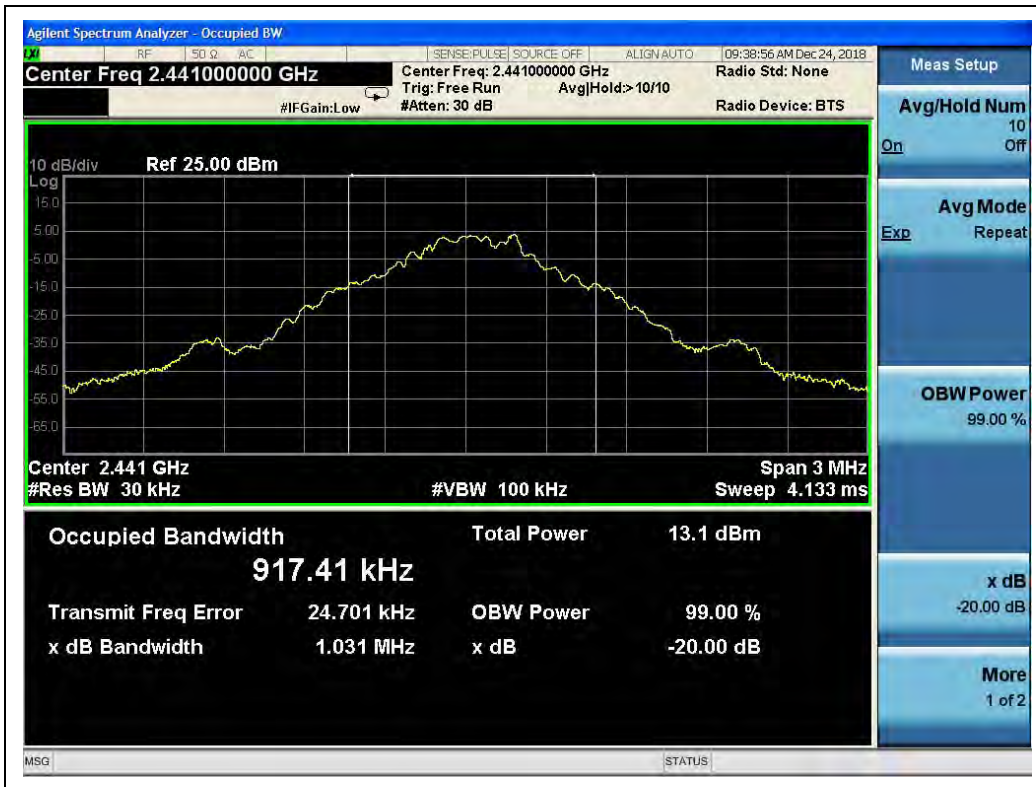
(GFSK, Channel 39, 2441MHz)
