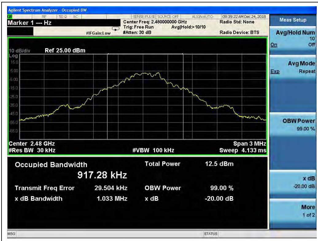
(GFSK, Channel 78, 2480MHz)
