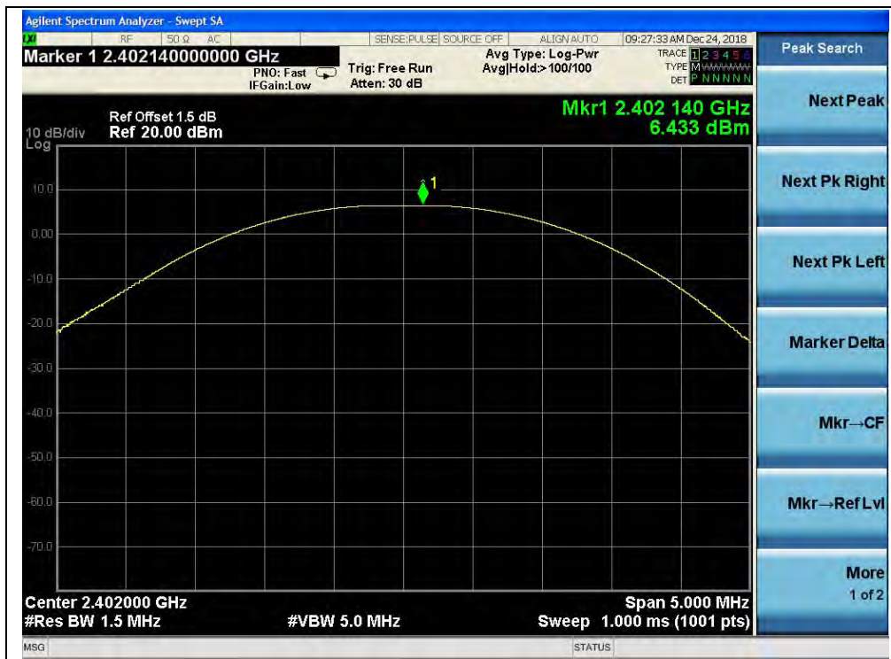
(GFSK, Channel 0, 2402MHz)
