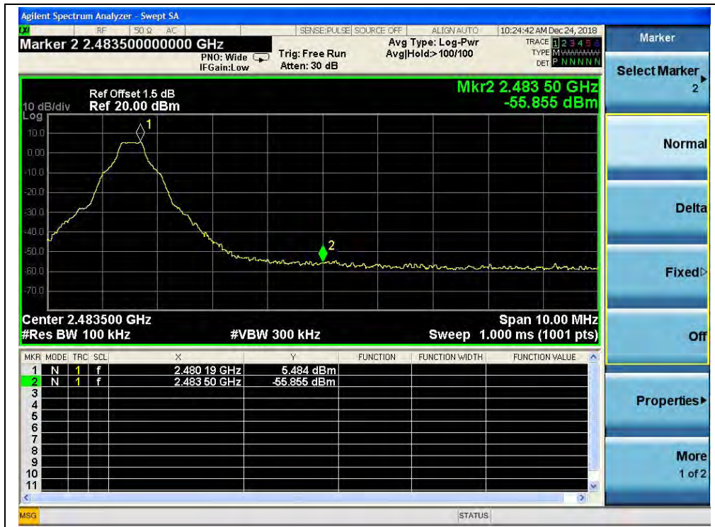
(Channel = 78, Band edge, GFSK Mode)
