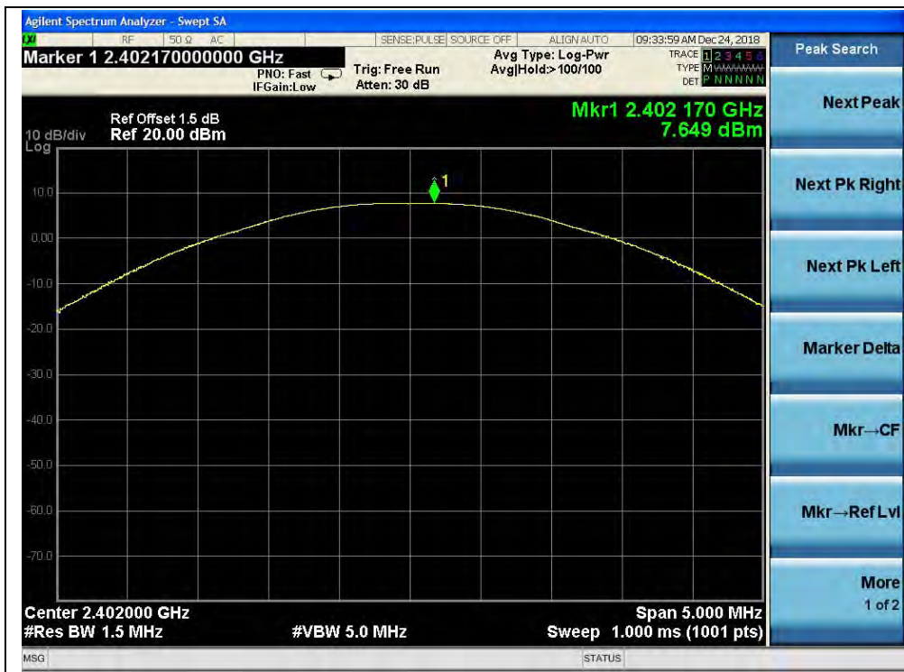
( \pi/4 -DQPSK, Channel 0, 2402MHz)
