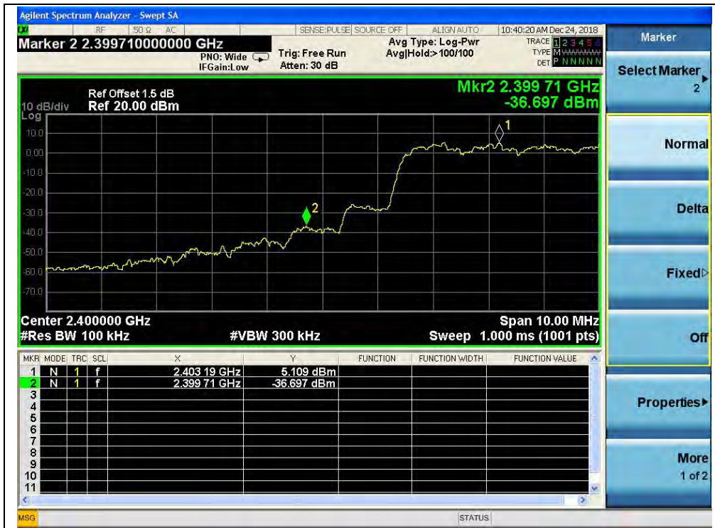
(Channel = 0, Band edge with hopping on, 8-DPSK)
