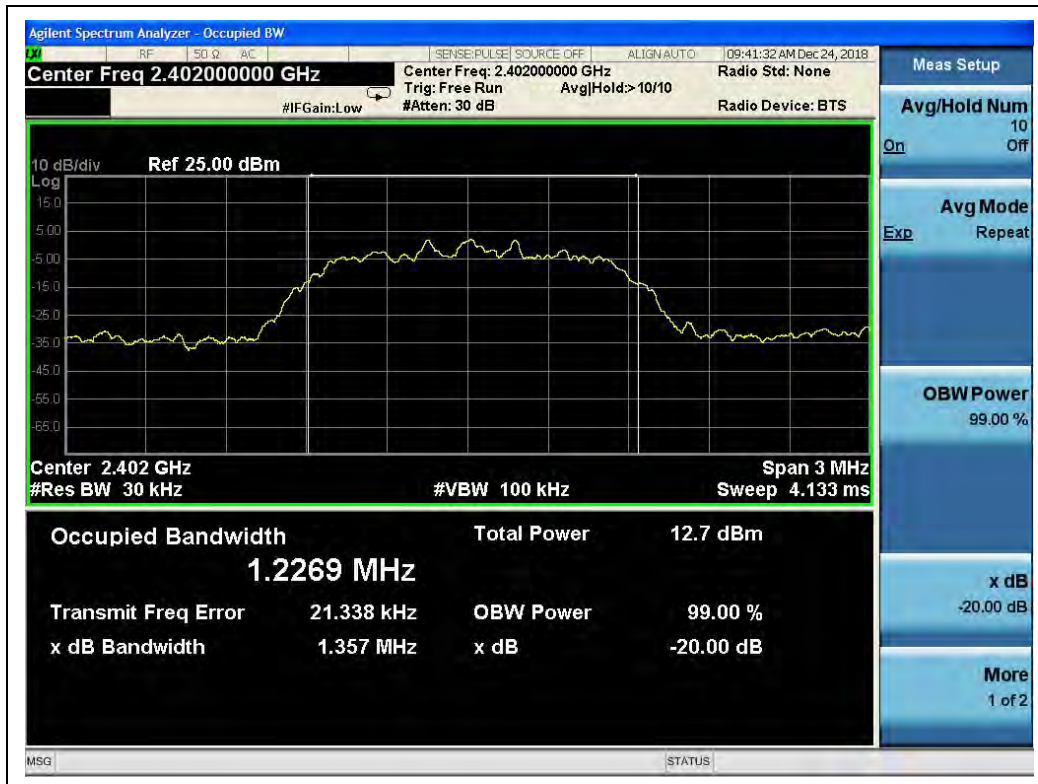
( \pi/4 -DQPSK, Channel 0, 2402MHz)
