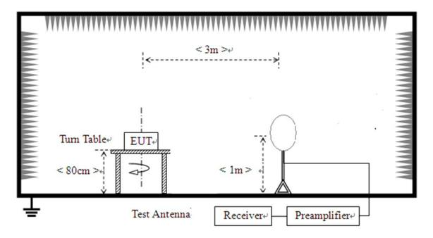
2) For radiated emissions from 30MHz to1GHz
