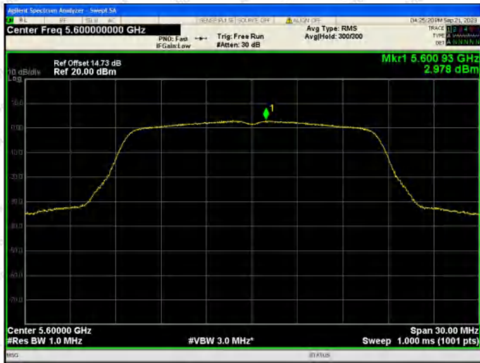
PSD NVNT a 5600MHz Ant1 SISO
