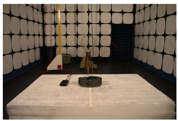
3. Radiated emission (9KHz-30MHz)
