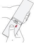
2 To replace the batteries, slide off the battery compartment backplate, insert new batteries (matching the polarity (+/-) as indicated), and close the battery compartment
