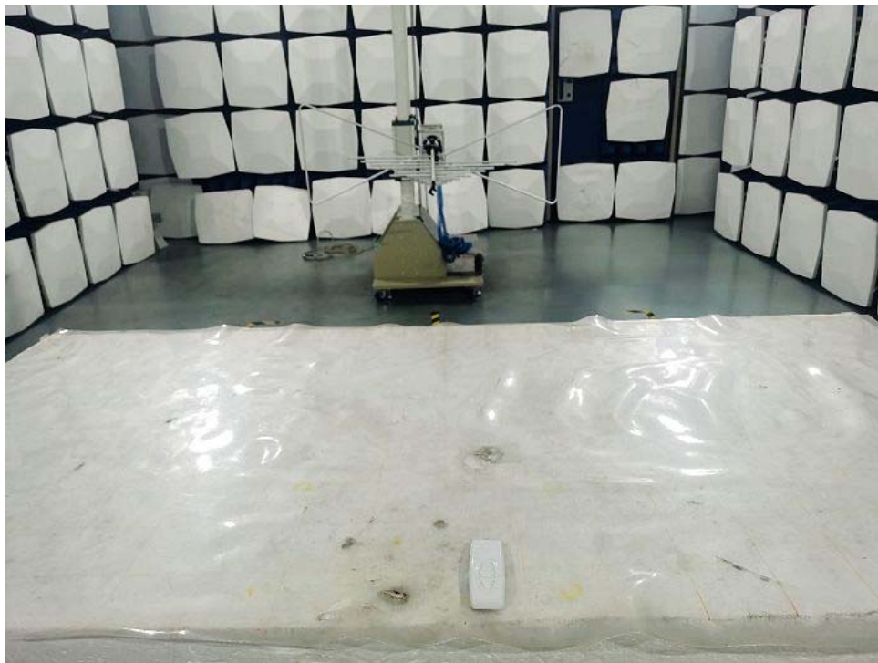
Radiated Emission Test Setup:
