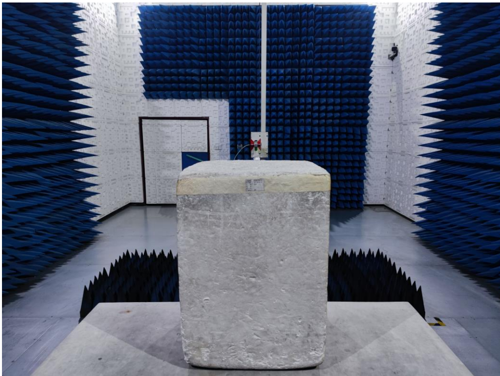
RADIATED EMISSION TEST SETUP ABOVE 1GHZ
