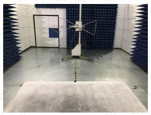
RADIATED EMISSION TEST SETUP ABOVE 1GHz
