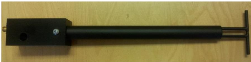
Figure 1 – MVG COMOSAR Validation Dipole
