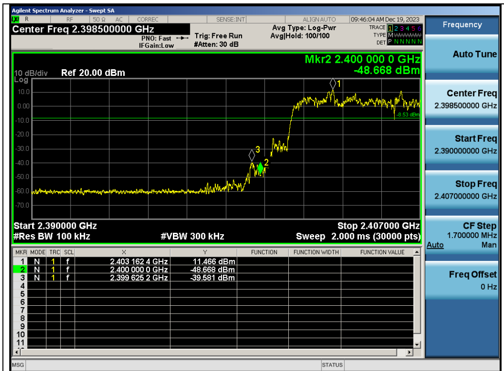
Test_Graph_EDR_HOP_ANT1_NA_3Mbps_Lower Band Edge Emissions
