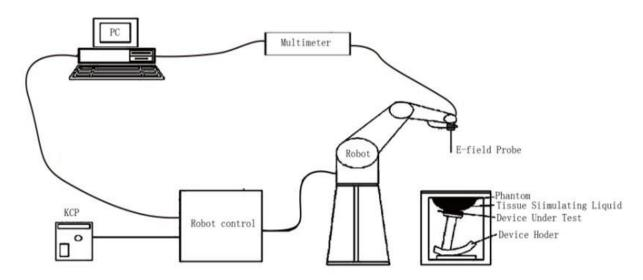
The COMOSAR system for performing compliance tests consists of the following items:
