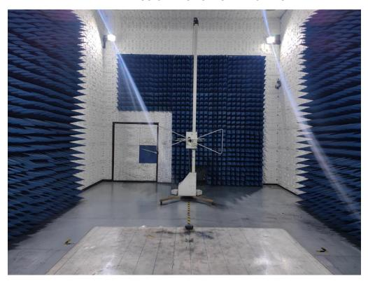
RADIATED EMISSION TEST SETUP ABOVE 1GHz
