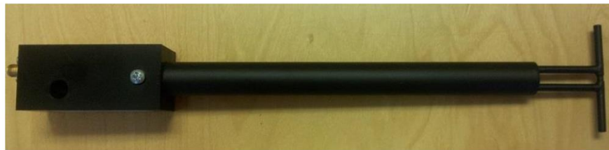
Figure 1 – MVG COMOSAR Validation Dipole
