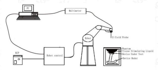
The COMOSAR system for performing compliance tests consists of the following items:
