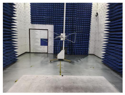
RADIATED EMISSION TEST SETUP ABOVE 1GHz
