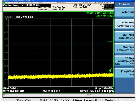
Test\_Graph\_LE1M\_ANT1\_2402\_1Mbps\_Lower Band Emissions
