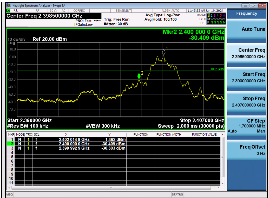
Test_Graph_LE2M_ANT1_2402_2Mbps_Lower Band Edge Emissions
