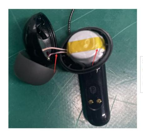
Speaker cable Battery cable twisted 3 turns, as shown in the figure (refer to project 2161B)
