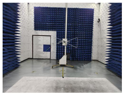
RADIATED EMISSION TEST SETUP ABOVE 1GHz
