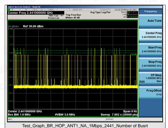
01:02:23 PM Apr 30, 2021 Trig Delay-2.000 ms Avg Type: Log-Pwr Trig: Video #Atten: 40 dB Center Freq 2.441000000 GHz PNO: Fast IFGain:Low
