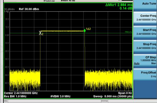
Test\_Graph\_BR\_HOP\_ANT1\_NA\_1Mbps\_2441\_Time per Burst
