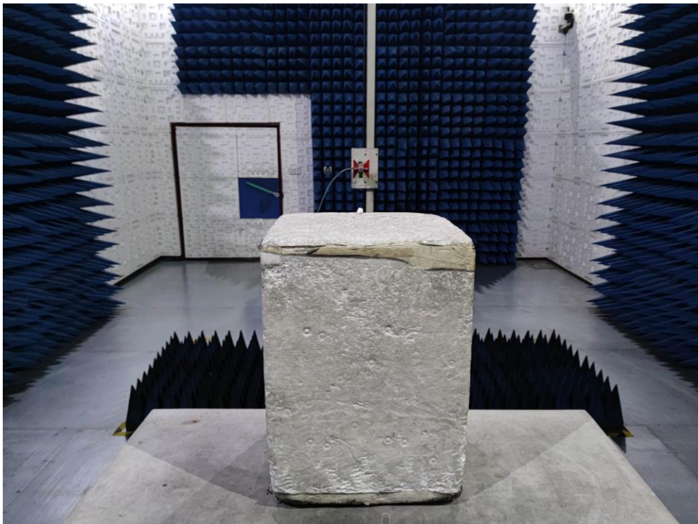
RADIATED EMISSION TEST SETUP ABOVE 1GHz
