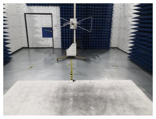
RADIATED EMISSION TEST SETUP ABOVE 1GHz
